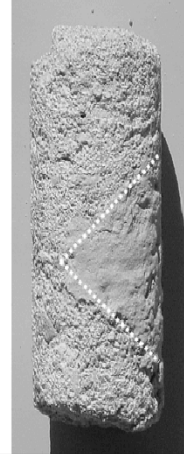
Rock core from the Ogallala Formation at F.E. Warren AFB illustrating a silt bed in sandstone
